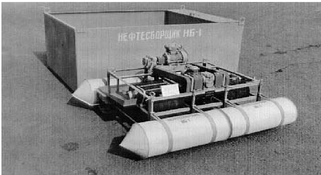
Fig.5. The series example of industrial swimming four-drum mechanize skimmer.
